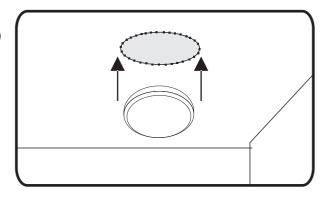
Step 3: Hold the two clips back against the panel light and push it into the hole. Allow the springs to pull the light up to the ceiling
